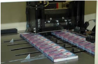
Photo 8 – quality control by machine inspection
